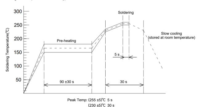
2. Recommended Hand Soldering Parameters
